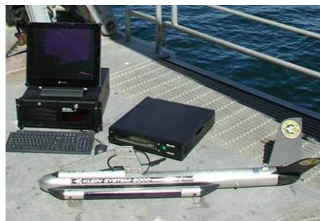
A side scan sonar towfish and related equipment.
