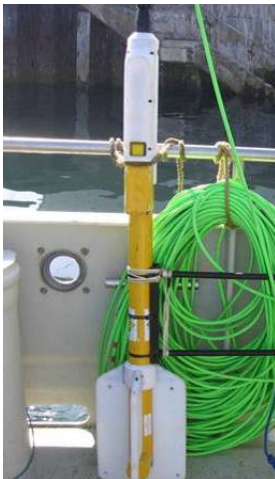
A magnetometer and its tether on the deck of a survey vessel. Image: OTF
